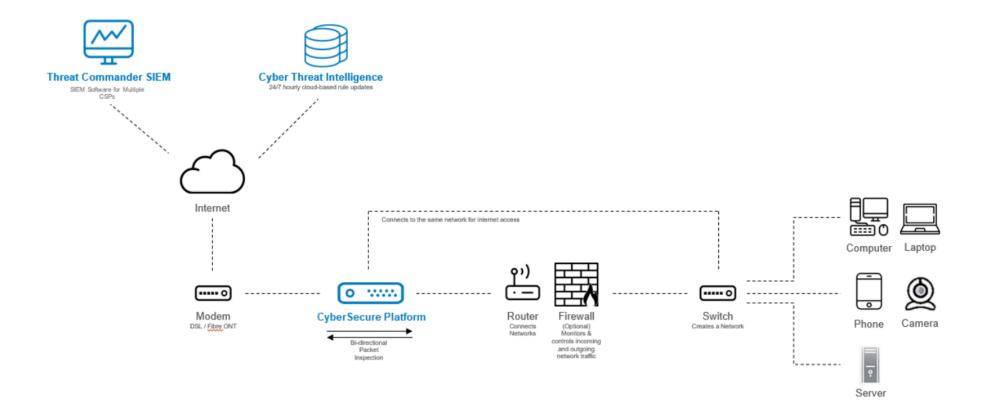
The CyberSecure Platform have been designed in a unique way that allows it to be installed in-line between an Internet router and a firewall, using modern cyber security techniques to protect a network from today's modern and sophisticated cyber-attacks by inspecting packets in real-time as they pass through the platform in both directions (inbound and outbound), at the same time dropping malicious packets before they have a chance to reach the internal network of the organization.
